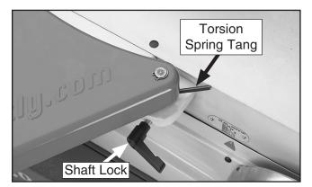
**Figure 60.** Guard mounted with spring tang in the correct position for proper return tension.
